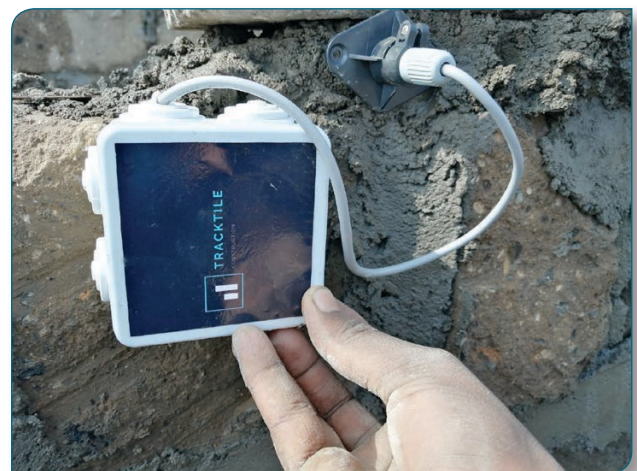
Tracktile measuring concrete on-site.
