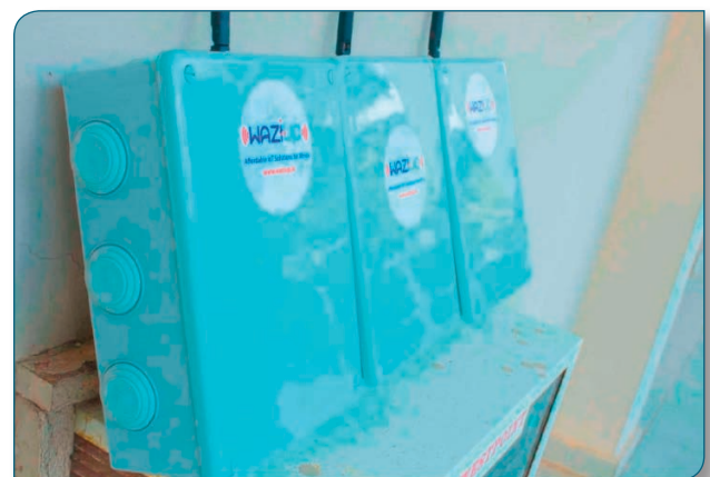
Our gateways ready to be deployed (Single channel low-cost LoRa gateway)
