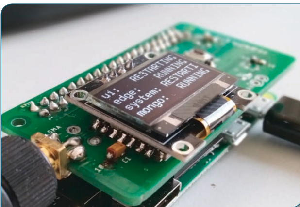
WaziHAT for multichannel LoRa with blackout protection circuit
